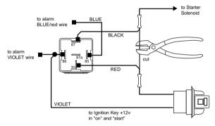
In this configuration, the vehicle will only start when the system is both connected and disarmed.
